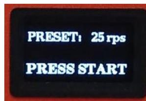
By turning the operating knob while the motor is running, the speed can be set to values between 5 and 200 rps. The desired speed is stored in non-volatile memory when the encoder button is pressed and is shown as preset value on the display. The display is dimmed during stand-by operation.
