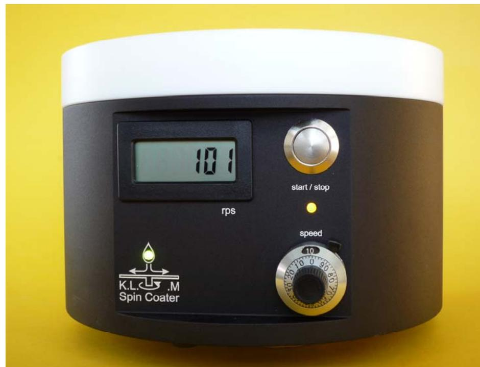
The fixing of the sample for SCV devices is carried out by an active vacuum pump. The vacuum pump can be connected by way of a quick release coupling on the back of the device, the sample will then be held in place during the coating process.
